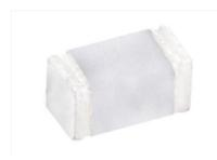
Gas discharge tubes (GDT) use noble gasses enclosed in ceramic tubes to provide an alternate circuit path for voltage spikes. The ceramic envelope and with nickel connectors allow for high loads and SURGING offers products that function at 20KA,40KA,50KA,60KA,100KA&150KA.The breakdown voltages of the devices have a wide range (up to 20% tolerance). Major applications are high frequency telecommunication lines, stations, security systems, HID and high quality Surge Protection Devices (SPD).
